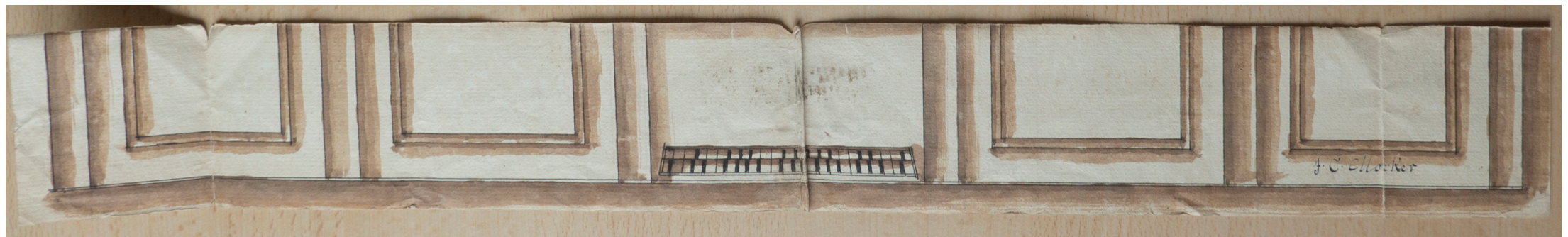
Details of the drawing: unfolding the lower part reveals the pedal board (below); a detail of the pedal board drawing is shown above. Note that the key C# was not planned for, as was usual in Hildebrandt's time and region.
