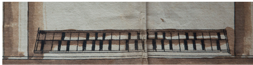
Details of the drawing: unfolding the lower part reveals the pedal board (below); a detail of the pedal board drawing is shown above. Note that the key C# was not planned for, as was usual in Hildebrandt's time and region.
