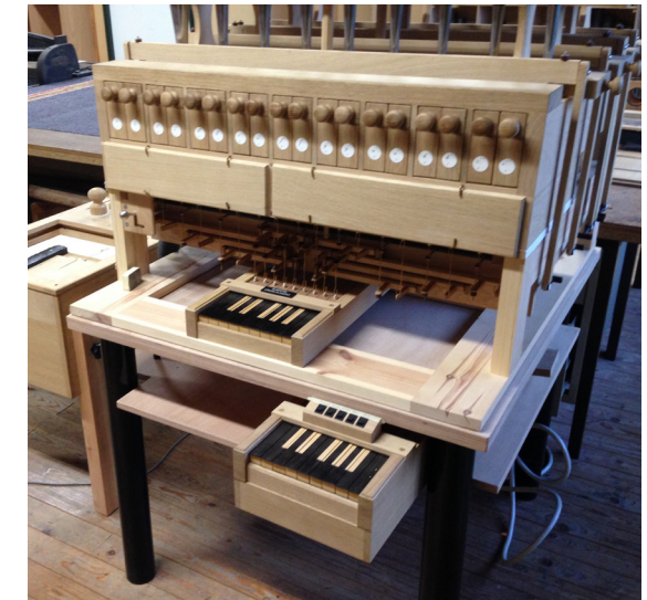
The test organ, built by Elbertse Orgelmakers, has a mechanical and a digital keyboard.
